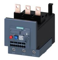
Overload relay 80...100 A Thermal For motor protection Size S3, Class 10 Contactor mounting Main circuit: Screw Auxiliary circuit: spring-type terminal Manual-Automatic-Reset
