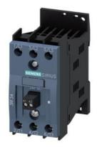
Solid-state contactor 3-phase 3RF3 AC 53 / 5.2 A / 40  $^{\circ}\text{C}$  48-480 V / 110-230 V AC 2-phase controlled Instantaneous switching screw terminal
