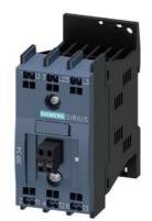
Solid-state contactor 3-phase 3RF3 AC 53 / 5.2 A / 40  $^\circ$ C 48-480 V / 110-230 V AC 2-phase controlled Instantaneous switching Spring-type terminal
