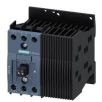
Solid-state contactor 3-phase 3RF3 AC 53 / 9.2 A / 40  $^\circ$ C 48-480 V / 24 V DC 2-phase controlled Instantaneous switching screw terminal
