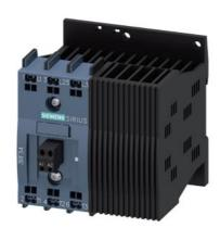
Solid-state contactor 3-phase 3RF3 AC 53 / 9.2 A / 40  $^{\circ}\text{C}$  48-480 V / 110-230 V AC 2-phase controlled Instantaneous switching Spring-type terminal
