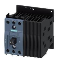
Solid-state contactor 3-phase 3RF3 AC 53 / 12.5 A / 40  $^{\circ}\text{C}$  48-480 V / 110-230 V AC 2-phase controlled Instantaneous switching screw terminal
