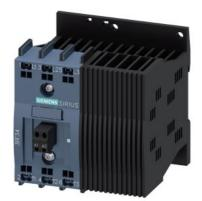
Solid-state contactor 3-phase 3RF3 AC 53 / 12.5 A / 40  $^\circ$ C 48-480 V / 110-230 V AC 2-phase controlled Instantaneous switching Spring-type terminal
