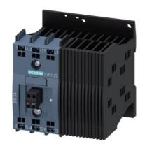
Solid-state contactor 3-phase 3RF3 AC 53 / 16 A / 40  $^{\circ}\text{C}$  48-480 V / 24 V DC 2-phase controlled Instantaneous switching Spring-type terminal
