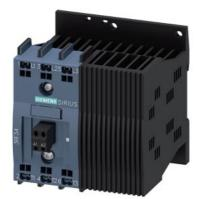
Solid-state contactor 3-phase 3RF3 AC 53 / 16 A / 40  $^\circ$ C 48-480 V / 110-230 V AC 2-phase controlled Instantaneous switching Spring-type terminal
