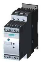
SIRIUS soft starter S0 32 A, 15 kW/400 V, 40  $^{\circ}\text{C}$  200-480 V AC, 110-230 V AC/DC Screw terminals
