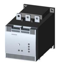
SIRIUS soft starter S12 280 A, 160 kW/400 V, 40 °C 200-460 V AC, 230 V AC Screw terminals !!! Phased-out product !!! Successor is SIRIUS 3RW5, Preferred successor type is >>3RW5074-6AB14<<
