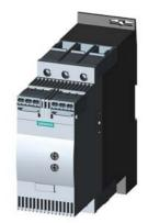
SIRIUS soft starter S2 63 A, 30 kW/400 V, 40  $^{\circ}\text{C}$  200-480 V AC, 24 V AC/DC spring-type terminals
