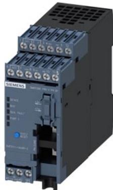
Basic unit SIMOCODE pro V PN GP Ethernet/PROFINET IO, PN system redundancy, OPC UA server, Web server, transmission rate 100 Mbps, 1 x bus connection via RJ45, 4 I/3 Q freely parameterizable, Us: 110...240 V AC/DC, input for thermistor connection Monostable relay outputs, expandable by 1 extension module(DM, TM, EM)
