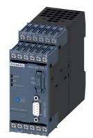
Basic unit SIMOCODE pro V MR, MODBUS RTU interface 57.6 Kbps, RS 485, 4I/30 freely parameterizable, Us: 110...240 V AC/DC, input for thermistor connection Monostable relay outputs, expandable by extension modules
