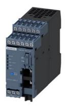
Basic unit SIMOCODE pro V EIP, EtherNet/IP, medium redundancy DLR, Web server, transmission rate 100 Mbps, 2 x bus connection via RJ45, 4I/3O freely parameterizable, Us: 24 V DC, input for thermistor connection Monostable relay outputs, expandable by extension modules
