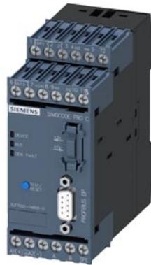
Basic unit SIMOCODE pro C, PROFIBUS DP interface 12 Mbit/s, RS 485, 4I/3O freely parameterizable, Us: 24 V DC, input for thermistor connection
