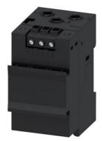
Current/voltage measuring module for dry-running protection of centrifugal pumps in hazardous areas; Set current 0.3 ... 4 A, Voltage measurement up to 690 V, width 45 mm, straight-through transformer
