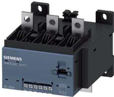
Current/voltage measuring module for dry-running protection of centrifugal pumps in hazardous areas; set current 20 ... 200 A, voltage measurement up to 690 V, width 120 mm, busbar connection
