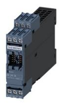
Digital module, 4 inputs and 2 relay outputs, input voltage 24 V DC, relay outputs bistable, max. 2 digital modules, for SIMOCODE pro V basic unit
