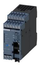
Basic unit SIMOCODE pro V PN GP , Ethernet/PROFINET IO, PN system redundancy, OPC UA server, Web server, transmission rate 100 Mbps, 2 x bus connection via RJ45, 4 l/3 Q freely parameterizable, Us: 24 V DC, input for thermistor connection Monostable relay outputs, expandable by 1 extension module(DM, TM, EM)
