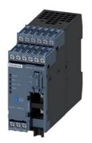
Basic unit SIMOCODE pro V PN GP , Ethernet/PROFINET IO, PN system redundancy, OPC UA server, Web server, transmission rate 100 Mbps, 1 x bus connection via RJ45, 4 l/3 Q freely parameterizable, Us: 24 V DC, input for thermistor connection Monostable relay outputs, expandable by 1 extension module(DM, TM, EM)
