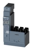
residual current device RCD510 Basic RCD type A side mounted rated resid. current 0.03...5A at 50/60Hz adjustable tv 0...3000ms 3-pole In=160A Ue=127-480V accessory for: 3VA1 with terminal connection
