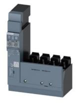
residual current device RCD510 Basic RCD type A side mounted rated resid. current 0.03...5A at 50/60Hz adjustable tv 0...3000ms 4-pole In=160A Ue=127-480V accessory for: 3VA1 with terminal connection
