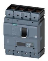
circuit breaker 3VA2 IEC frame 630 breaking capacity class M Icu=55kA @ 415V 4-pole, line protection ETU850, LSI, In=500A overload protection Ir=200A...500A short-circuit protection Isd=0.6..10x In, Ii=1.5..14x In N conductor protection adjustable (OFF, up to 100%) nut keeper kit
