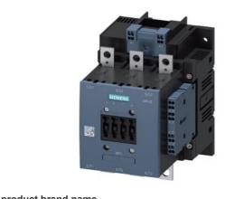
Power contactor, AC-3 150 A, 75 kW / 400 V AC (50-60 Hz) / DC operation 23-26 V UC Auxiliary contacts 2 NO + 2 NC 3-pole, Size S6 Busbar connections Drive: conventional Spring-type terminal
