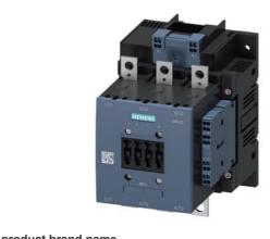
Power contactor, AC-3 150 A, 75 kW / 400 V AC (50-60 Hz) / DC operation 110-127 V UC Auxiliary contacts 2 NO + 2 NC 3-pole, Size S6 Busbar connections Drive: conventional Spring-type terminal
