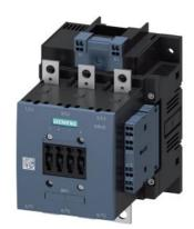
Power contactor, AC-3 150 A, 75 kW / 400 V AC (50-60 Hz) / DC operation 220-240 V UC Auxiliary contacts 2 NO + 2 NC 3-pole, Size S6 Busbar connections Drive: conventional Spring-type terminal
