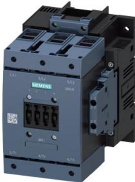
Power contactor, AC-3 150 A, 75 kW / 400 V AC (50-60 Hz) / DC operation 23-26 V UC Auxiliary contacts 2 NO + 2 NC 3-pole, Size S6 Busbar connections Operating mechanism: conventional Screw terminal Box terminal block 3RT1955-4G mounted
