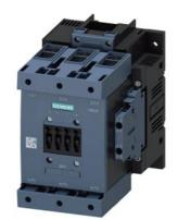
Power contactor, AC-3 185 A, 90 kW / 400 V AC (50-60 Hz) / DC operation 23-26 V UC Auxiliary contacts 2 NO + 2 NC 3-pole, Size S6E Busbar connections Drive: conventional with 2 box terminals 3RT19 56-4G up to 120 mm
