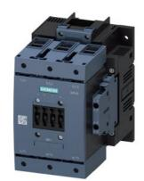
Power contactor, AC-3 185 A, 90 kW / 400 V AC (50-60 Hz) / DC operation 23-26 V UC Auxiliary contacts 2 NO + 2 NC 3-pole, Size S6E Busbar connections Drive: conventional with 2 box terminals 3RT19 55-4G up to 70 mm
