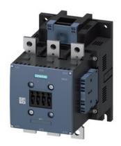
Power contactor, AC-3 225 A, 110 kW / 400 V AC (50-60 Hz) / DC operation 23-26 V UC Auxiliary contacts 2 NO + 2 NC 3-pole, Size S10 Busbar connections Drive: conventional Spring-type terminal
