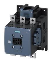
Power contactor, AC-3 225 A, 110 kW / 400 V AC (50-60 Hz) / DC operation 110-127 V UC Auxiliary contacts 2 NO + 2 NC 3-pole, Size S10 Busbar connections Drive: conventional screw terminal
