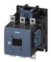
Power contactor, AC-3 300 A, 160 kW / 400 V AC (50-60 Hz) / DC operation 23-26 V UC Auxiliary contacts 2 NO + 2 NC 3-pole, Size S10 Busbar connections Drive: conventional Spring-type terminal
