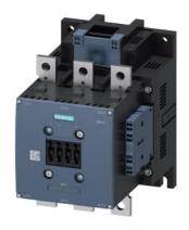
Power contactor, AC-3 300 A, 160 kW / 400 V AC (50-60 Hz) / DC operation 110-127 V UC Auxiliary contacts 2 NO + 2 NC 3-pole, Size S10 Busbar connections Drive: conventional Spring-type terminal
