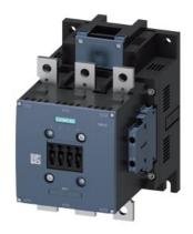
Power contactor, AC-3 300 A, 160 kW / 400 V AC (50-60 Hz) / DC operation 220-240 V UC Auxiliary contacts 2 NO + 2 NC 3-pole, Size S10 Busbar connections Drive: conventional screw terminal
