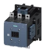
Power contactor, AC-3 400 A, 200 kW / 400 V AC (50-60 Hz) / DC operation 23-26 V UC Auxiliary contacts 2 NO + 2 NC 3-pole, Size S12 Busbar connections Drive: conventional Spring-type terminal
