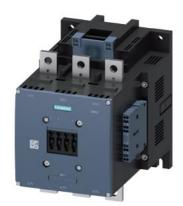
Power contactor, AC-3 400 A, 200 kW / 400 V AC (50-60 Hz) / DC operation 110-127 V UC Auxiliary contacts 2 NO + 2 NC 3-pole, Size S12 Busbar connections Drive: conventional Spring-type terminal
