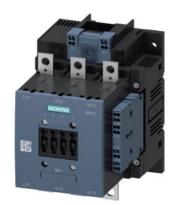
Power contactor, AC-3 115 A, 55 kW / 400 V AC (50-60 Hz) / DC operation 110-127 V UC Auxiliary contacts 2 NO + 2 NC 3-pole, Size S6 Busbar connections Drive: conventional Spring-type terminal
