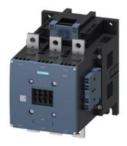
Power contactor, AC-3 500 A, 250 kW / 400 V AC (50-60 Hz) / DC 23-26 V UC Auxiliary contacts 2 NO + 2 NC 3-pole, size S12 Busbar connections Operating mechanism: conventional Spring-type terminals
