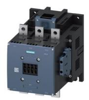
Power contactor, AC-3 500 A, 250 kW / 400 V AC (50-60 Hz) / DC 110-127 V UC Auxiliary contacts 2 NO + 2 NC 3-pole, size S12 Busbar connections Operating mechanism: conventional screw terminals
