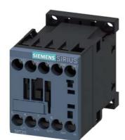
Power contactor, AC-3 7 A, 3 kW / 400 V 1 NC, 110 V AC, 50 / 60 Hz 3-pole, Size S00 screw terminal
