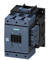
Power contactor, AC-3 115 A, 55 kW / 400 V AC (50-60 Hz) / DC operation 23-26 V UC Auxiliary contacts 2 NO + 2 NC 3-pole, Size S6 with box terminals Drive: conventional Spring-type terminal
