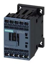
Power contactor, AC-3 7 A, 3 kW / 400 V 1 NO, 110 V AC, 50/60 Hz 3-pole, Size S00 Spring-type terminal
