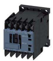
Power contactor, AC-3 7 A, 3 kW / 400 V 1 NO, 24 V AC, 50 Hz 3-pole, Size S00 ring cable lug connection
