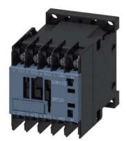
Power contactor, AC-3 7 A, 3 kW / 400 V 1 NO, 220 V AC, 50 Hz 240 V, 60 Hz, 3-pole, Size S00, ring cable lug connection
