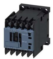
Power contactor, AC-3 7 A, 3 kW / 400 V 1 NC, 220 V AC, 50 Hz 240 V, 60 Hz, 3-pole, Size S00, ring cable lug connection
