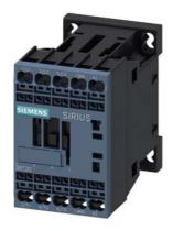
Power contactor, AC-3 9 A, 4 kW / 400 V 1 NO, 24 V AC, 50 / 60 Hz, 3-pole, Size S00 Spring-type terminal
