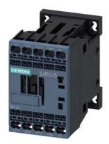
Power contactor, AC-3 9 A, 4 kW / 400 V 1 NO, 110 V AC, 50/60 Hz 3-pole, Size S00 Spring-type terminal
