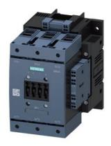
Power contactor, AC-3 115 A, 55 kW / 400 V AC (50-60 Hz) / DC operation 220-240 V UC Auxiliary contacts 2 NO + 2 NC 3-pole, Size S6 with box terminals Drive: conventional Spring-type terminal
