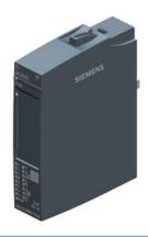
SIPLUS ET 200SP, digital input modul, DI 8x DC 24V SRC BA, -40...+70°C with conformal coating based on 6ES7131-6BF61-0AA0 . type 1 (IEC 61131), source Input (NPN, M-reading) Packing unit: 1 piece, fits to BU-type A0, Colour Code CC02, input delay time 0,05..20ms, module diagnostics for: supply voltage
